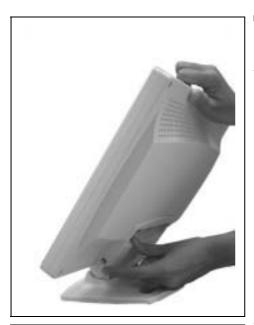
Hold the monitor base firmly with one hand and carefully tilt the display upwards with the other hand.
