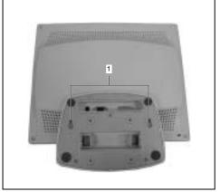
Place the display over the screws so that the screws slot into the mounting holes (1) in the monitor base and lock into place.
