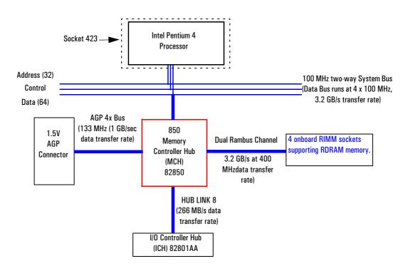
The supported operating frequency of the AGTL+ bus for the Pentium 4 is 100 MHz. The width of the data bus is 64 bits, while the width of the address is 32 bits. Data bus transfers occur at four times the system bus, at 400 MHz. Along with the operating frequencies, the processor voltage is set automatically.
