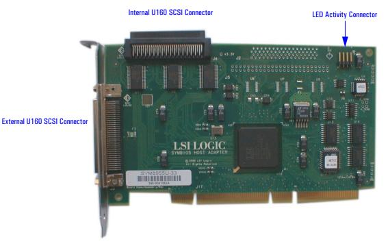
The functionality and performance of the Ultra 160 SCSI PCI Adapter card comes from the on-board LSI Logic SYM53C1010 PCI to Ultra 160 multifunction controller with LVD link universal transceivers.
