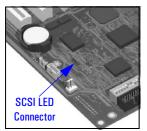
The LED cable supplies SCSI LED activity to the front panel hard disk LED. For this to work, the SCSI LED cable must be connected to the LED Activity connector on the Ultra 160 SCSI PCI Adapter card (refer to graphic on page <u>87</u>) and the SCSI LED connector on the system board.
