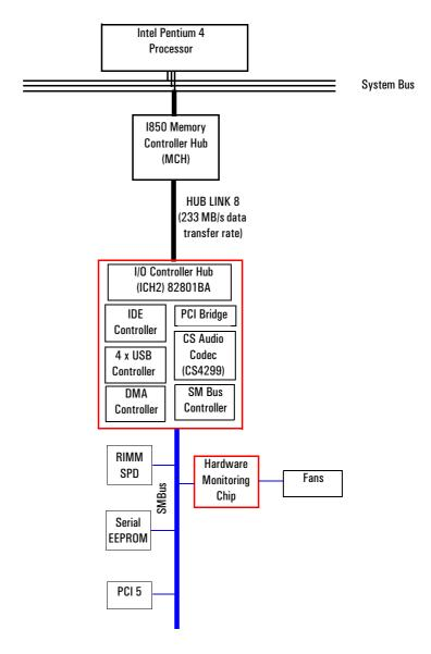
The Input/Output Controller Hub 2 (82801BA)
