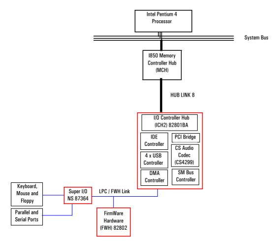
The Input/Output Controller Hub 2 (82801BA)
