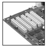
There is a total of five Peripheral Component Interconnect (PCI) 32-bit, 33 MHz connectors on the system board.
