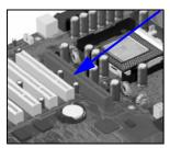
Minitower models of the HP Vectra VL800 are equipped with a single AGP (Accelerated Graphics Port) graphics slot.
