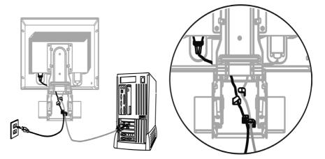
e. Put the stand cover (e) back then put the cable cover (f) back.
